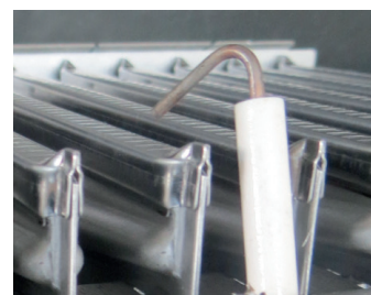
Electrode assembled on the manifold side
